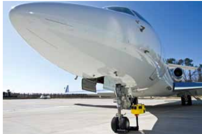
Vigiplane installed on front landing gear of Dassault Falcon 7x
